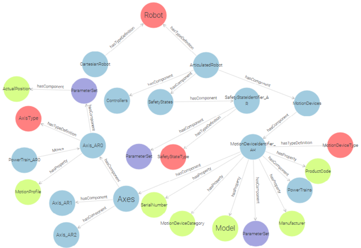
Fig. 7. Simplified visualization of the Robotics knowledge graph
