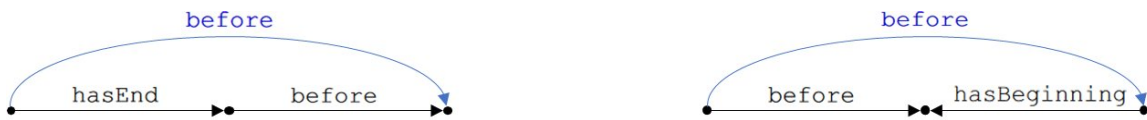
Fig. 10. Inferences on the property before ; the inferred properties are shown in blue.
