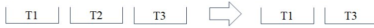
Fig. 3. Transitivity of Before : if T1 occurs before T2 and T2 occurs before T3 , then T1 occurs before T3 .
