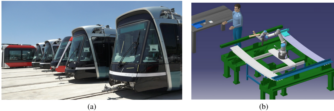
Figure 9. Design of the collaborative cell of the RAILWAYS scenario to support workers in the assembly of door frames.
