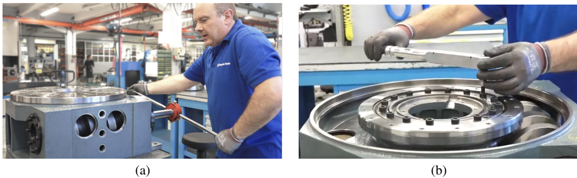
Figure 8. Working area of the CAPITAL-GOODS scenario (a) and structure of the workpiece (b) where a collaborative robot is deployed to support workers in repetitive screwing/unscrewing tasks.
