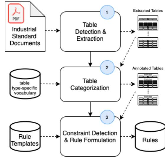
Fig. 12. Process of extracting constraints from tables.
